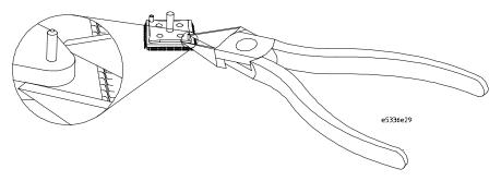
**3** Ensure that the tip edge of the plier is as nearly parallel as possible and resting on the surface of the TQFP.
