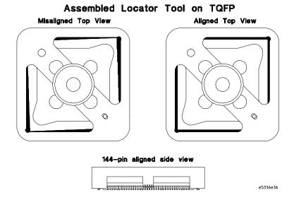
**3** Press down on the middle of both sides of the locator tool. If the tool is down far enough, it will not rock when pressed on the sides.
