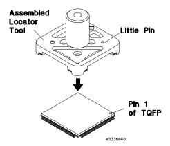
2 Place the assembled locator tool on the TQFP, making sure that it aligns squarely. You will feel the teeth drop between the TQFP legs when it is aligned.
