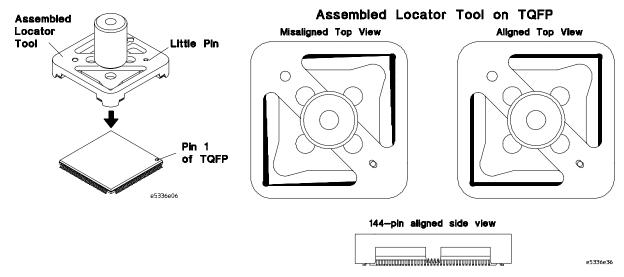
3 Hold down on the sides of the locator tool and loosen the knurled nut two turns. Continue to hold down on the sides of the locator tool and press down on the knurled nut to drop the retainer onto the top of the TQFP. Hold for 45 seconds.
