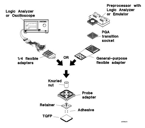
This Installation Guide explains how to use Hewlett-Packard's advanced probing system for 0.5 mm pitch Thin Quad Flat Pack (TQFP) surface-mounted integrated circuits. This probing system provides a quick and reliable connection from these devices to Hewlett-Packard oscilloscopes, logic analyzers, and emulators.
