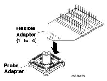
**5** Connect the appropriate logic analyzer or oscilloscope probe to the correct circuit as indicated by the adapter pin numbers.
